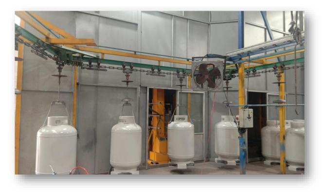
Powder Coating Line for Large LPG Cylinder, Factory 4
